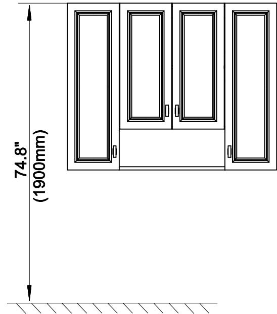
Draw the spacing between the walls and the No.10, punch holes in the wall, and fix the No.10 to the wall with screws.
